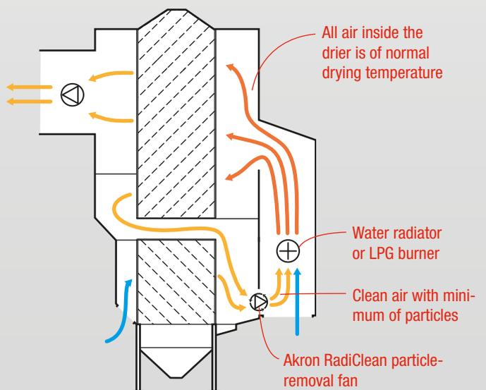
**Akron Svegma RC drier with active particle reduction.** With Akron's RadiClean fan, air can be recirculated before the heating arrangement. Heating only needs to be performed to the required drying temperature, which allows for other heating options. No air mixing inside the drier is necessary.
