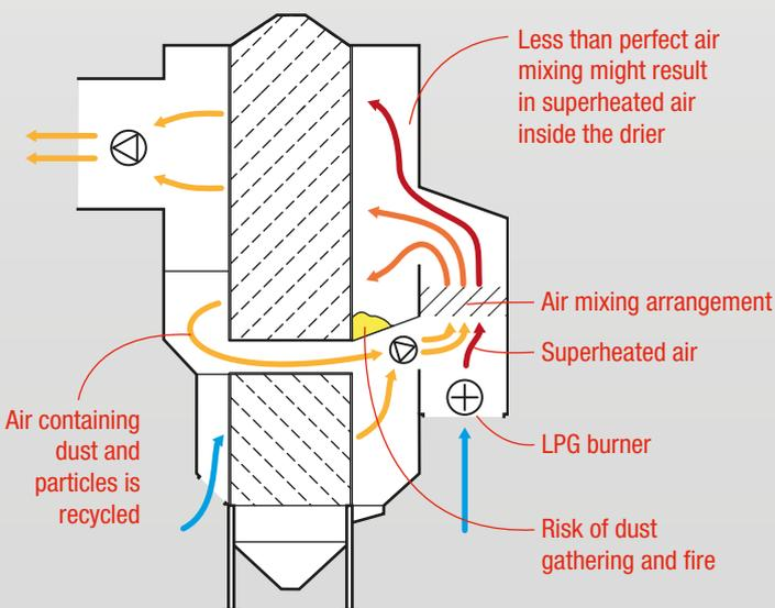
**Traditional recirculation drier.** The air is recirculated after the heating arrangement. To achieve the correct drying temperature it must be mixed with superheated fresh air. Due to this, almost all traditional recirculation driers are heated with LPG. Efficient mixing of the air is required for even drying.
